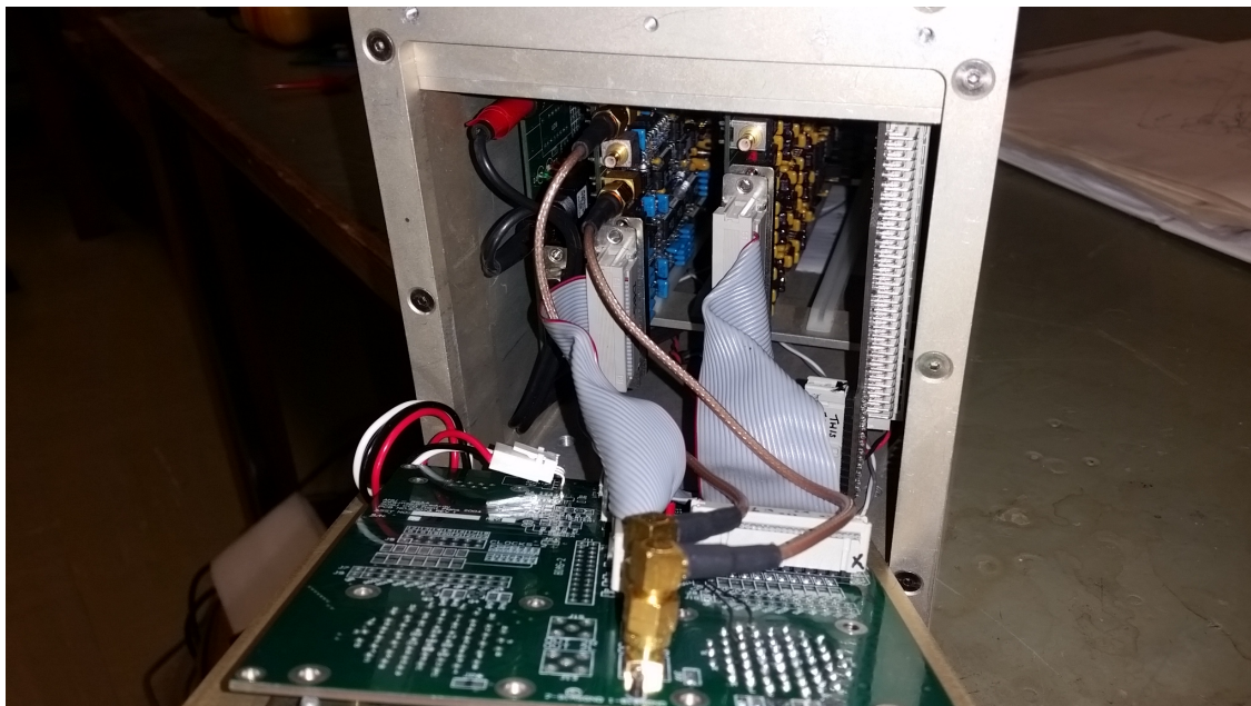
Figure 4: End view showing card layout and connectors
